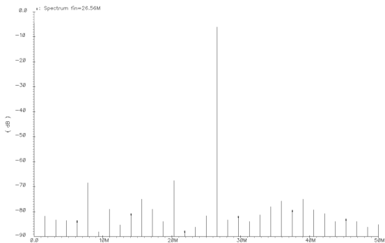
Fig.7 FFT spectrum when f_{in}=26.56\text{MHz}
